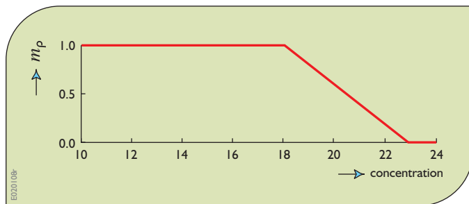
Figure 5.13. Membership function for 'about 20 mg/l or less'.
