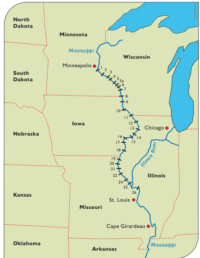
Figure D.19. The upper Mississippi River locks and navigation dams, known locally as pools.
